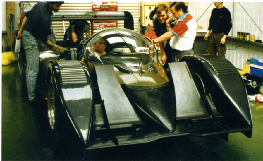
Front wing design, with its secondary flaps between the wings, was way ahead of its time, and worked too
