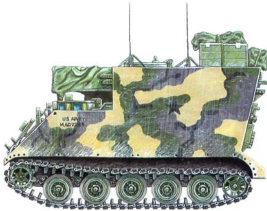
G1: M577A1 command post vehicle of 3-112 Armor, 49th Armored Division (Texas National Guard); Oklahoma, summer 1999.
