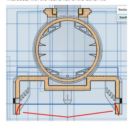
Also note, the lower leading and trailing edge will need some rounding, again in order to accommodate the donor kit's round hull:
