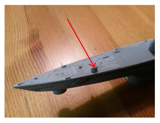
The main bow sonar dome (the large one below the torpedo tubes) again required some filing to get it to match the shape of the hull. Once attached, some putty filler (I'm a fan of Tamiya's) was needed in order to smooth out the transition:
