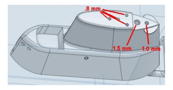
Conning tower placement, centered and 25.5 mm rearwards of the previously used point.
